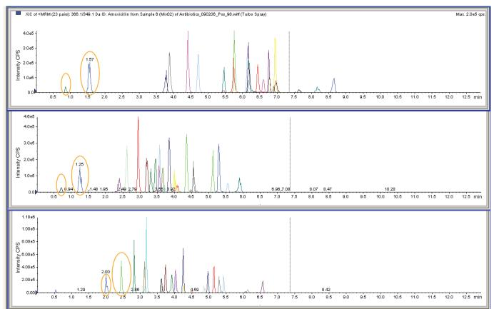
Column screening provides critical information leading to selection of the Kinetex<sup>™</sup> core-shell C18 column. The core-shell particle provides longer retention of the compounds of interest. Narrow Peak width, on Kinetex<sup>™</sup> core-shell C18 produces higher peak intensities.
