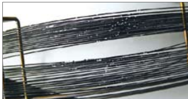
Figure 1. Traditional capillary columns easily break with prolonged exposure to GC oven temperatures above 360 °C.
